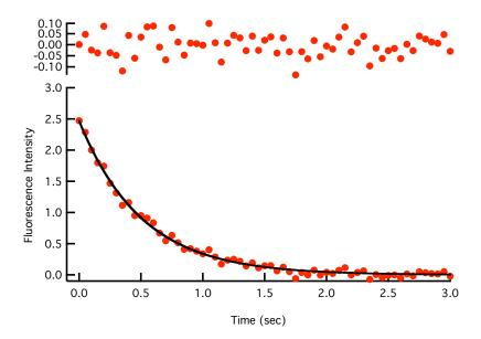
Note that the distribution of the residuals is the same across the entire fitted region, indicating that the fit is excellent and the distribution of the residuals is totally random. The width of the residuals reflects the Gaussian noise in the original "data" which we synthesized. The standard deviation of the residuals is about 0.05 (the value used in the gnoise function above).
